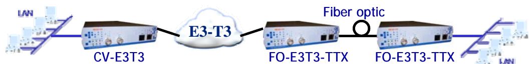
Ethernet interconnection through an E3 or T3 link
